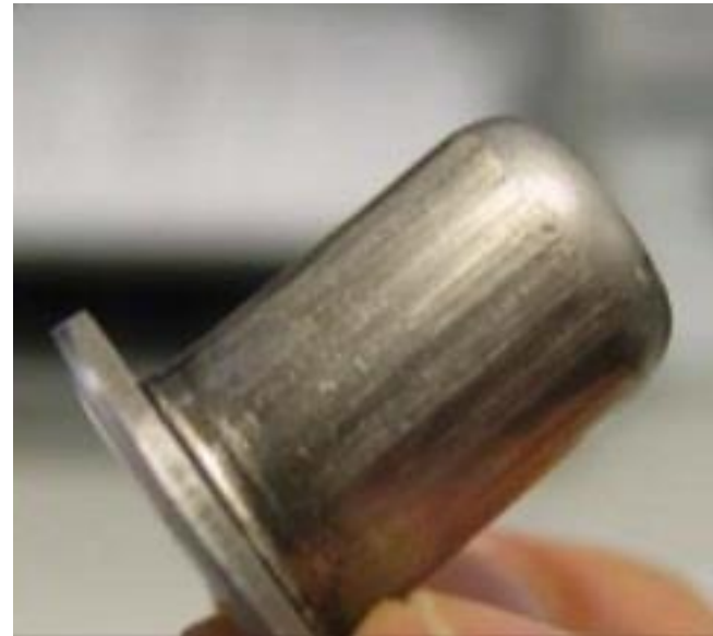
Fig. 1. Deep drawn component, (a) good surface quality, (b) poor quality due to galling
